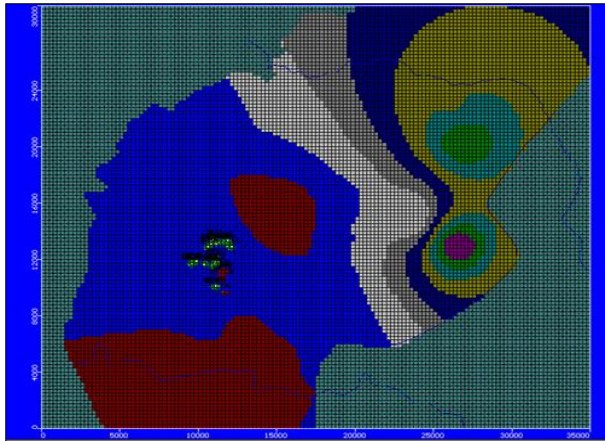
Fig. 06: The Hydraulic conductivity raster map processed in ArcGIS with use of available data
